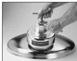
2) Insert the T-Wrench into the nut of the Poppet.
